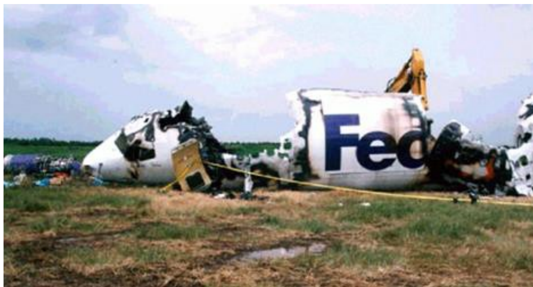
Figure 16. Federal Express – Boeing – B727-232F (N-497FE) flight FX1478. 29 The crash left several crew members injured and destroyed the aircraft. The National Transportation and Safety Board determined the pilot was not able to recognize the precision approach path indicator (PAPI) lights due to his color vision deficiency, which may have been exacerbated by stress and fatigue.
