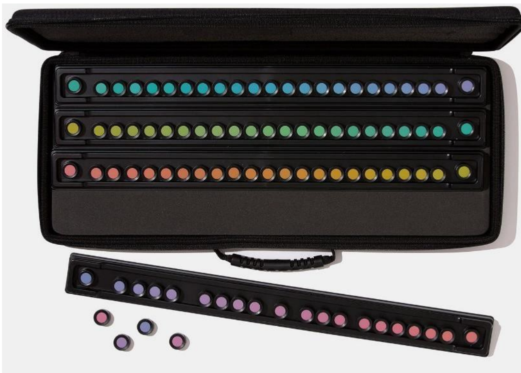
Figure 21. FM-100 Hue. 37 There are 85 caps in the test with anchor caps at each end of the box. The subject is asked to arrange the caps by hue.
