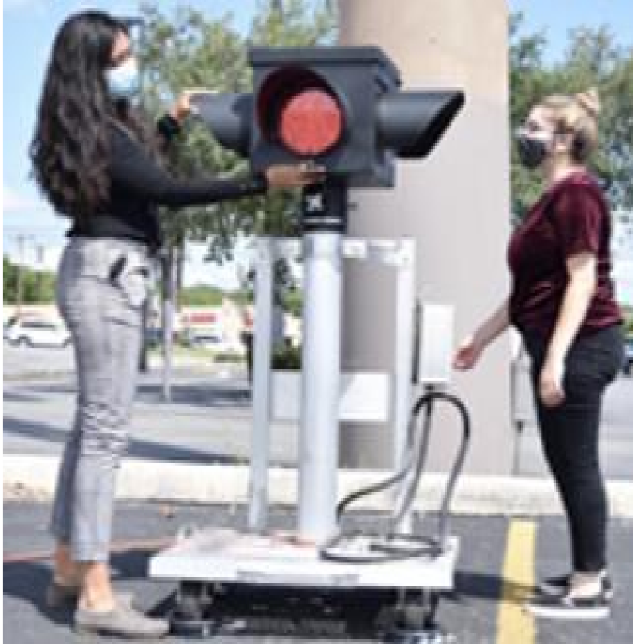
Figure 31. New Signal Light Test. The signal light on top of the pole rotates to display either a red light (shown above), green light, white light, or yellow light.
